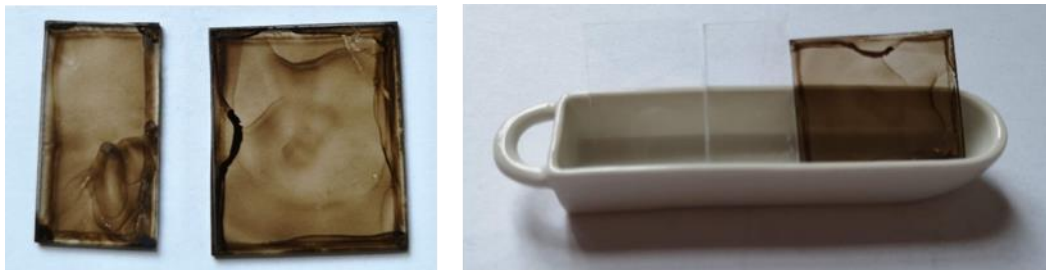
Figure 26 – Samples obtained after heat treatment in hydrogen conditions (on left) and the transparent color obtained after room atmosphere treatment.
